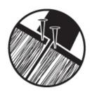
3. Thatch strips are cut in the middle of the corner rafters and secured by nails. Step 5 will cover any gaps.
