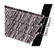
2. Then each strip is to be nailed 80mm apart. Pre-mark the rafters in 80mm increments. Place the next strip above the first strip and nail the second bamboo batten 80mm from the first bamboo batten. The layering effect at 80mm increments is critical to make the thatch roof waterproof.
