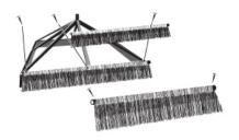
1. Begin the layering process of the thatch strips at the bottom of the roof structure, adjacent to the fascia. Nail through the bamboo batten to the rafters using either a nailgun or hammer.
